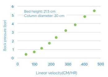
**Fig.7.** Efficiency of column (20 id x 21.5 cm high) packed with polymethacrylate based media
