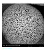
The average pore size of the beads is 500 A, providing on exclusion limit of  $1x10^6$  Dalton
