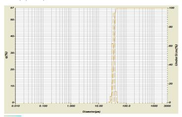
A median particle size of 35 micron and a particle size distribution of less than 1.4  $(d_{60}/d_{10})$  show a lack of fines and result in high efficiency at low back pressure.
