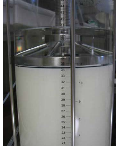
Fig.8. Polymeric media packed in a 200/500 Glass Column
