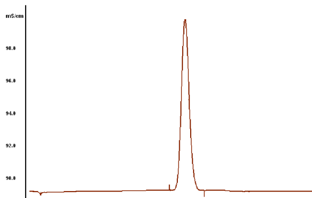
Fig. 11. Efficiency of column (45 cm id x 18 cm high) packed with PolyABx
